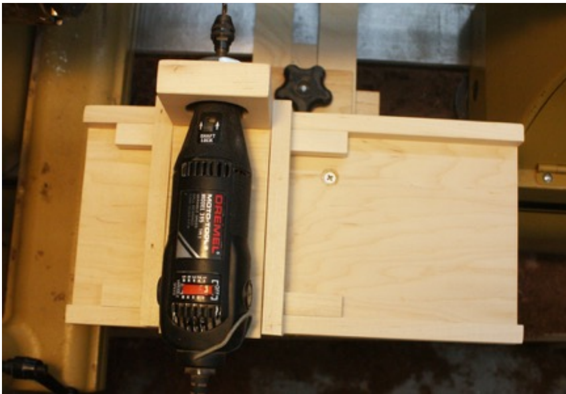
Top view of sled and Dremel in its holder. The sled can be clamped in place if just one hole is to be drilled for each leg.
