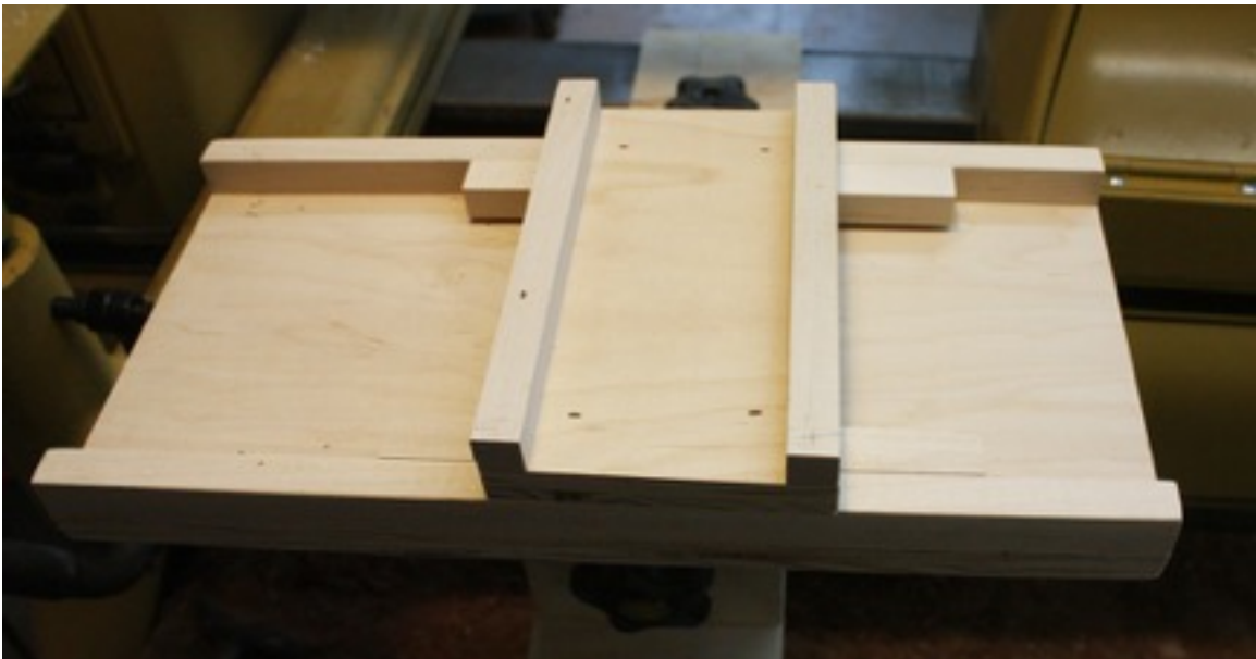
The sled that holds the Dremel tool. The sled slides sideways for drilling multiple parallel holes. The platform is 12" wide and the sled will travel around 8".
