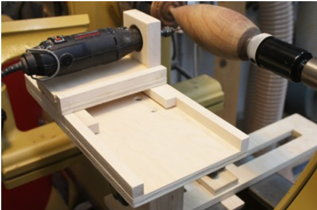
The sled with the Dremel in its holder. The holder slides forward to drill the holes in the vessel.
