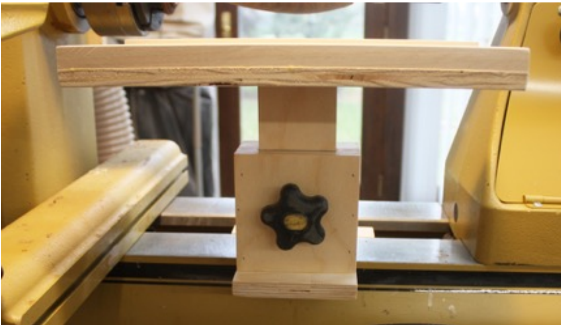
End view of platform showing locking knob for the support column. The column can travel vertically several inches to accommodate different sizes of lathes.
