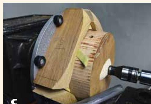
*Shims are used to adjust the position while centering the blank. The jaw's buttons visible here were used only as an aid in setting up each of the four wasteblocks, providing a reference point until the blocks were mounted with screws. The buttons are not involved in holding the wooden extensions in place. Note the protective scrap wood between the live center and the blank. The tailstock can be removed to allow access for light, final shaping cuts.*
