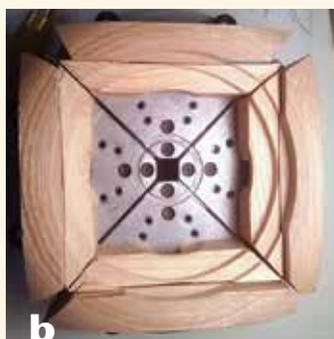
*Jumbo, flat, or Cole chuck jaws outfitted with custom-turned extension blocks can hold the disk blank. These accessory jaws are screwed in from the back of the chuck jaws but could also be screwed from the front with countersunk holes.*
